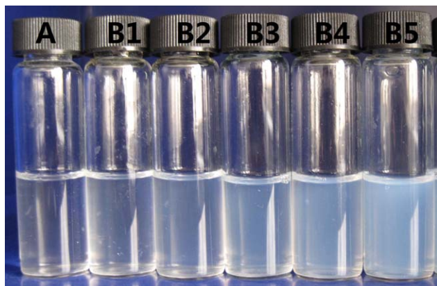
Figure 4. Appearances of HAPAM (A) and HAPAM/silica hybrid (B) in pure water ( T = 25^\circ\text{C} ) with different silica loading: (B1) 0.5 wt %, (B2) 1.0 wt %, (B3) 1.5 wt %, (B4) 2.0 wt %, and (B5) 2.5 wt %. [Color figure can be viewed in the online issue, which is available at wileyonlinelibrary.com .]
